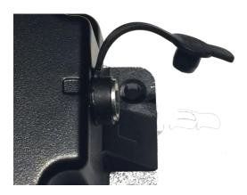
3. Once the Slap "N" Track Mini is fully charged (red LED on charger turns dim green) push the rubber weatherproof cap all the way into the charging port. This will ensure that moisture and dirt will not get into the charging port.
