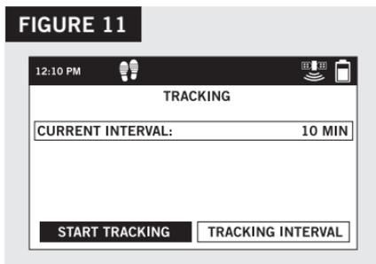
2. Once your GPS position is acquired, SPOT X will send your tracks in accordance with the tracking interval you have selected until you manually stop tracking, the SPOT X detects no movement, or you power off the SPOT X device.
